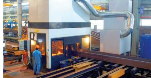
3D CNC OXYGEN & PLASMA CUTTING LINE FOR BEAMS DÂY CHUYỀN CẮT DÀM 3D CNC OXYGEN & PLASMA
